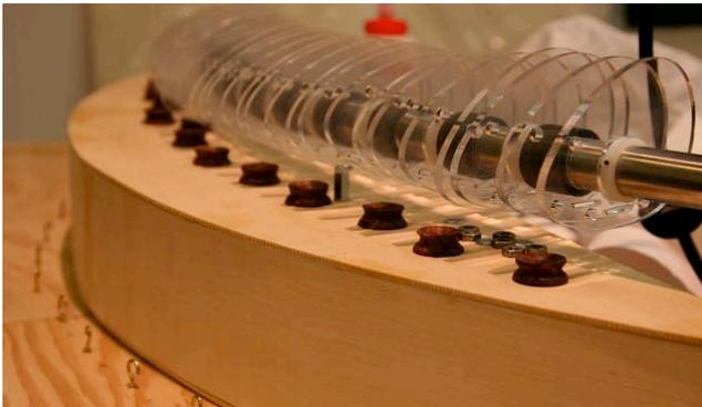
**Figure 3. Rose Wood Bridges Transfer The Vibrations**
