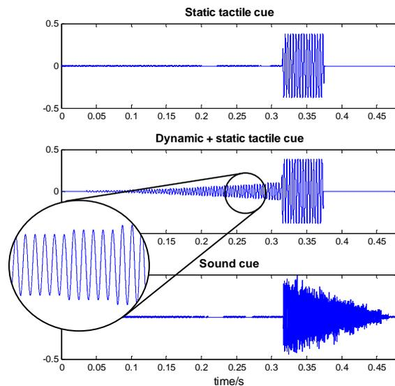
**Figure 1.** The tactile and sound signals triggered when crossing the virtual control surface. The illustration reflects a strike occurring with a velocity of 60°/s. The virtual control surface is crossed at 0.32 seconds.
