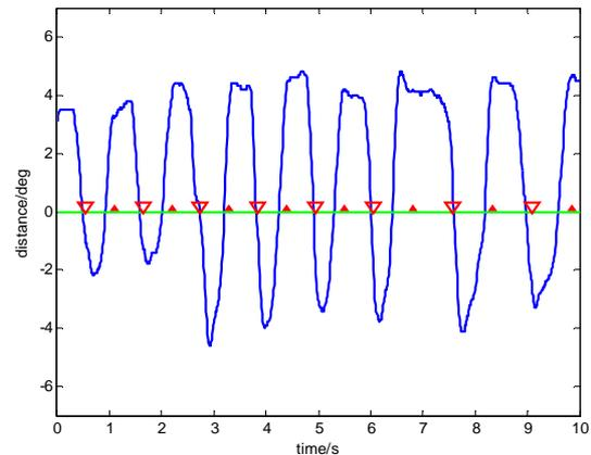
**Figure 3.** An example of experiment session output data. The bigger downward pointing triangles represent the higher beeps of the tempo sequence while small triangles the lower beeps. The task of the player was to strike at the higher beeps. The vertical axis represents the distance to the virtual control surface. The successful strokes are the zero crossings of the declining curve.
