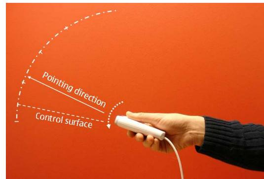
**Figure 2.** Playing the virtual instrument was based on a virtual control surface that was struck with sensor-actuator device. When the tilt angle of the device crossed the control surface, a percussive sound was triggered
