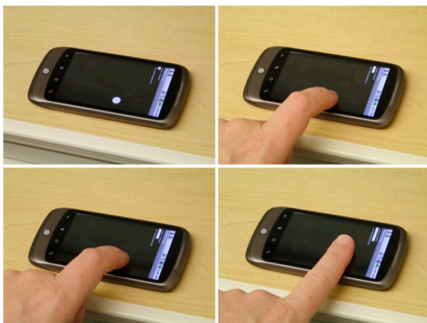
Figure 5 - Four distinct pressure levels on a Nexus One Android phone. Minimal pressure (top left), light pressure (top right), strong pressure (bottom left), flat finger (bottom right).
