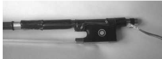
Figure 1: Picture of the bow mounted pressure sensors, after ca. 3000 played bowing samples.
